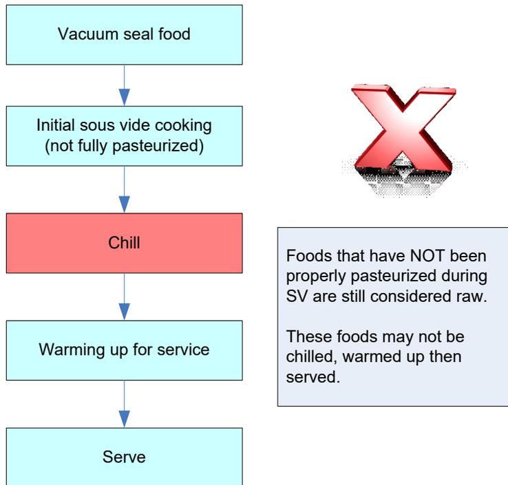
**Figure 9 – Interrupted sous vide process**
